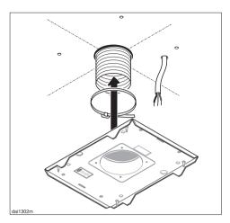
■ Secure the ducting to the mounting plate using a hose clip.
